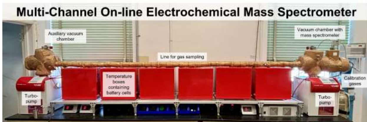
Figure 1. Multi-channel OEMS for quantification of gases in battery cells during cycling.
