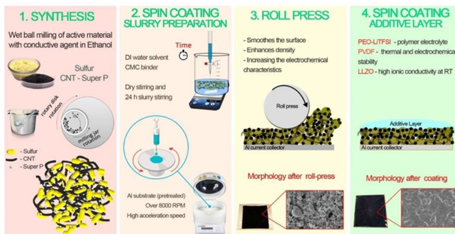
Figure 1. Schematic representation of cathode preparation
